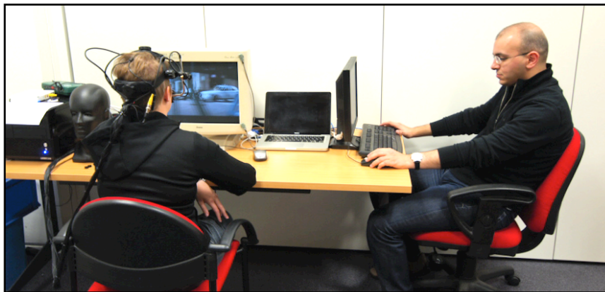
Figure 2. Experimental setup. The viewer watched the videos on a CRT monitor while wearing a head mounted eye tracking device. The experimenter ran the experiment from a non-intrusive position.
