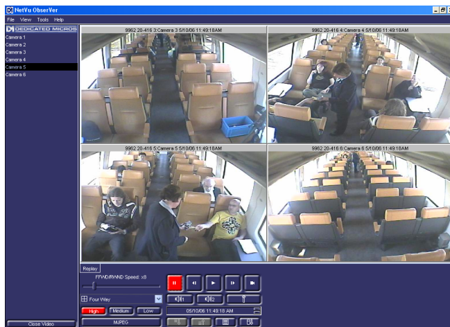
Figure 14.4.1 User interface for train compartment surveillance operator.
