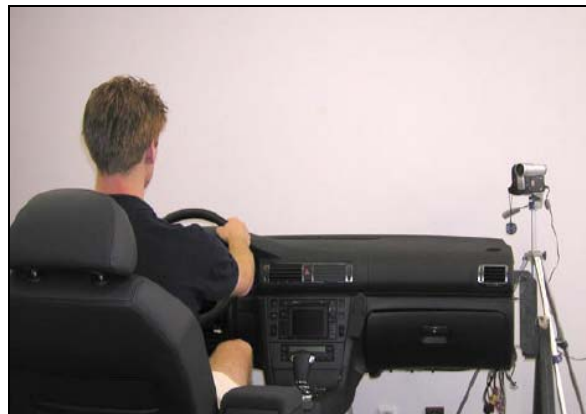
Fig. 1: Experimental setup for multimodal emotion recognition in car environment
