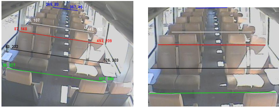
Fig. 3. Lines known to lie parallel to the x -axis can be used for determination of \phi (left). Validation of the result: after rotation in the reverse angle, all the chosen lines are approximately horizontal (right)
