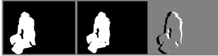
Fig. 3: (a) Silhouette frame image i (b) Silhouette frame image i+1. (c) Frame differencing.
