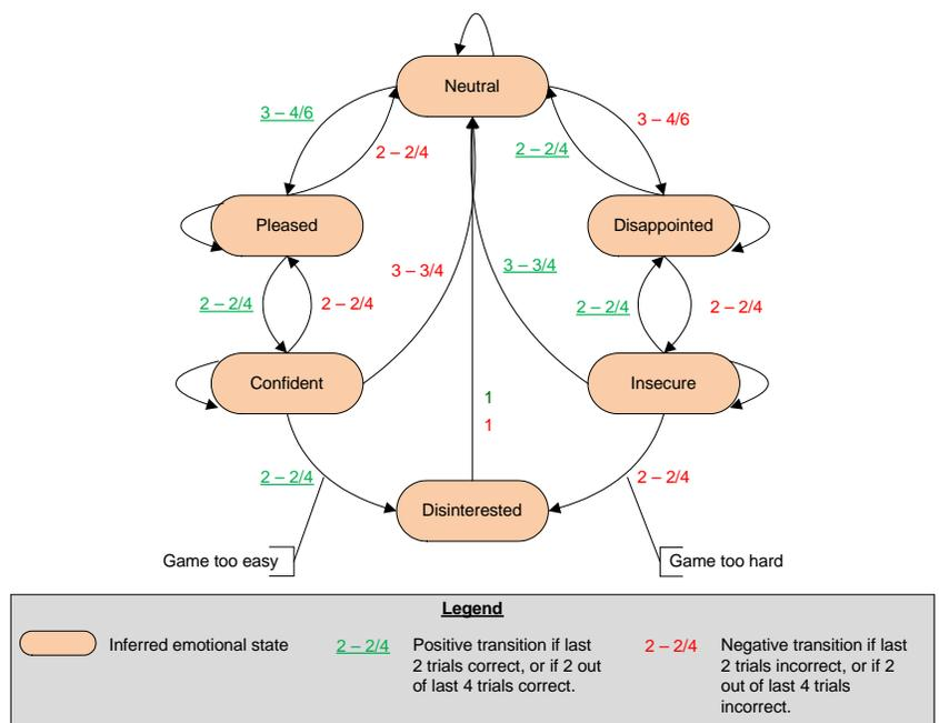
Figure 9 - Emotion knowledge base and the transitions triggered by semantic primitives for the input controller
