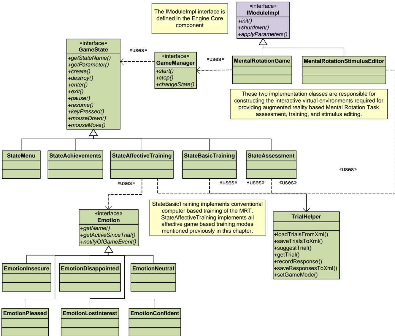
Figure 32 - High level overview of the Thesis Base component
