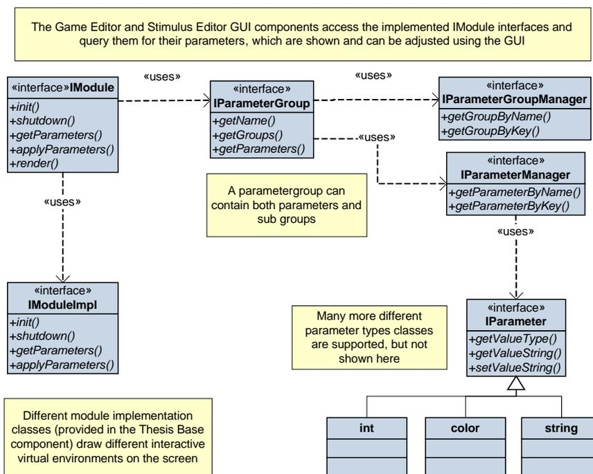
Figure 31 - High level overview of the Engine Core component
