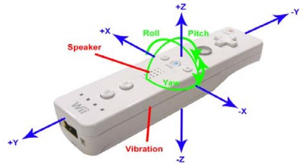
Figure 6 - Input sensors and output actuators of the Nintendo Wii Remote
