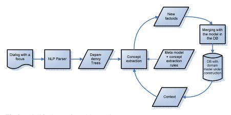
Fig. 1. Method for Automatic Model Extraction
