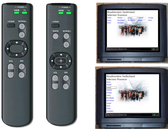
Figure 6: (left) linear-oriented remote control; (middle) plane-oriented remote control; (right upper corner) matrix layout; (right lower corner) list layout.
